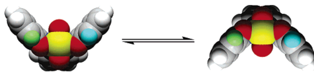
FIGURE 1. Flipping motion of compound 2a . The calculated structures are observed from the equatorial plane of the uranyl unit. The blue and green hydrogen atoms differentiate the two otherwise indistinguishable conformations.
